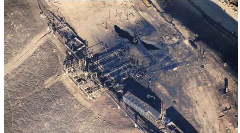
SS-25 site showing 60x40x20 ft deep vent.
